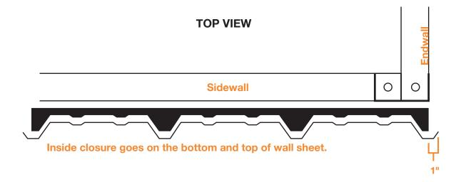
NOTE: Start sheets 1" in from corner channel and start sheet 1" above the bottom of the base channel.
