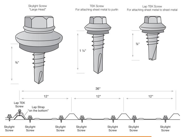
NOTE: Make sure to use TEK screws to attach sheets to purlins, lap TEK screws to attach sheets to sheets.
