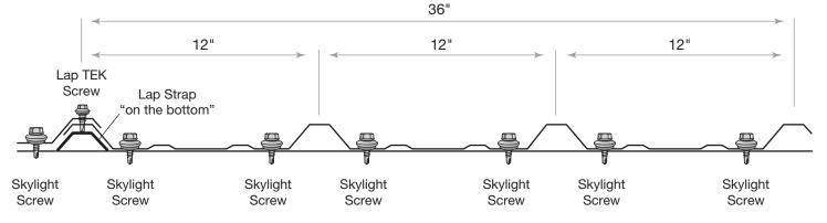
NOTE: Make sure to use TEK screws to attach sheets to purlins, lap TEK screws to attach sheets to sheets.
