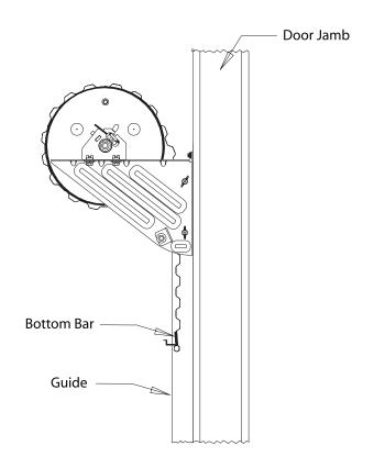
■ Install the Slide Lock with hardware provided. Optional on L250. Standard on M250.
