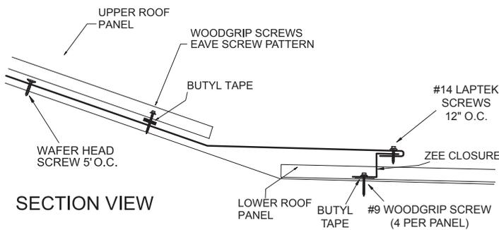
**NOTE: TO COMPLY WITH TEXAS WINDSTORM CERTIFICATION TESTING, #12X11 SDT TYPE A SCREWS MUST BE USED IN PLACE OF THE #9 WOODGRIP SCREWS.**
