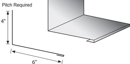
**Endwall to Roof Flashing CW**
