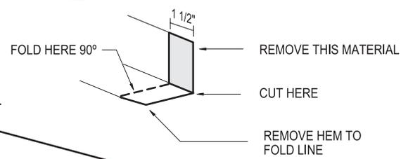
1. Trim both ends of the uphill and downhill sides of the flashing as indicated.
