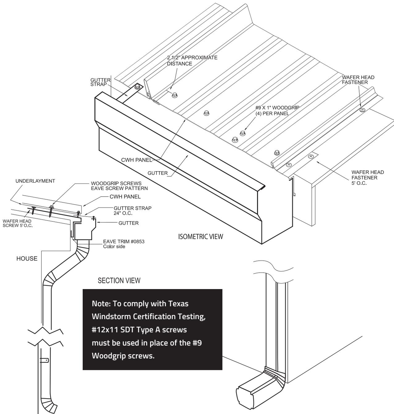
**Note:** To comply with Texas Windstorm Certification Testing, #12x11 SDT Type A screws must be used in place of the #9 Woodgrip screws.
