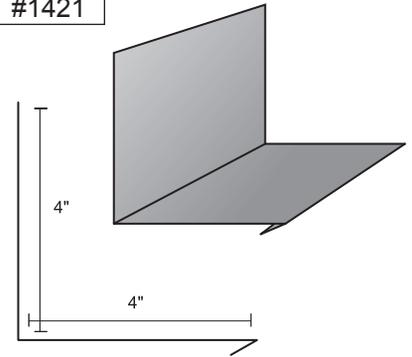
**Endwall to Roof Flashing**
