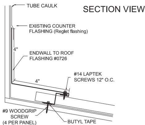
**NOTE: TO COMPLY WITH TEXAS WINDSTORM CERTIFICATION TESTING, #12X11 SDT TYPE A SCREWS MUST BE USED IN PLACE OF THE #9 WOODGRIP SCREWS.**
