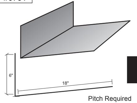
**Chimney Flashing Side**
