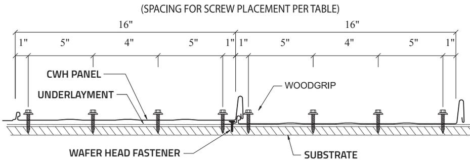
**Note:** To comply with Texas Windstorm Certification Testing, #12x11 SDT Type A screws must be used in place of the #9 Woodgrip screws.
