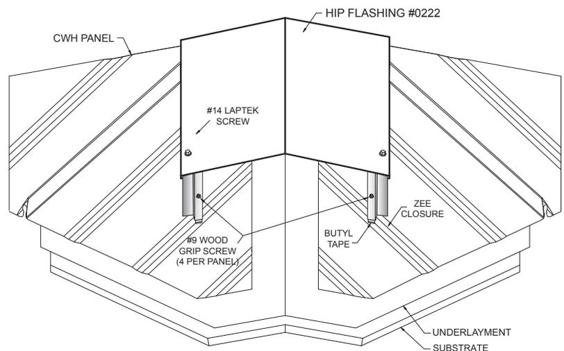
**Note:** To comply with Texas Windstorm Certification Testing, #12x11 SDT Type A screws must be used in place of the #9 Woodgrip screws.
