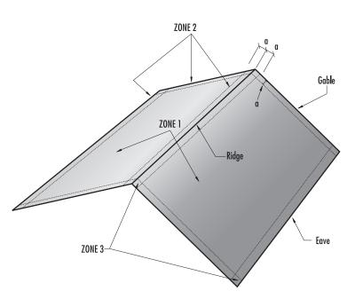
Note: Dimension (a) is defined as 10% of the minimum width of the building or 40% of the mean height of the roof, whichever is smaller, however, (a) cannot be less than either 4% of the minimum width of the building or 3 feet.
