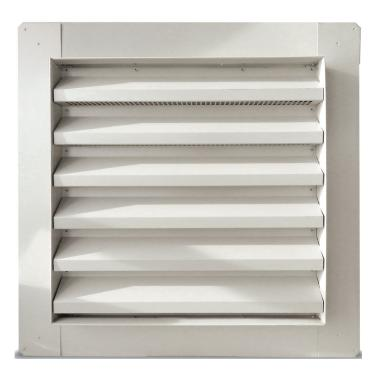
Cut and trim opening to appropriate Vent / Opening size. Use pop rivets to hold trim in place. Insert vent into opening from inside of building until vent flange meets the trim. Attach vent from outside of building using screws long enough to penetrate through wall sheet, trim and into the flange on the vent. Caulk as required where trim meets the vent flange. Trim, fasteners and caulk not included.
