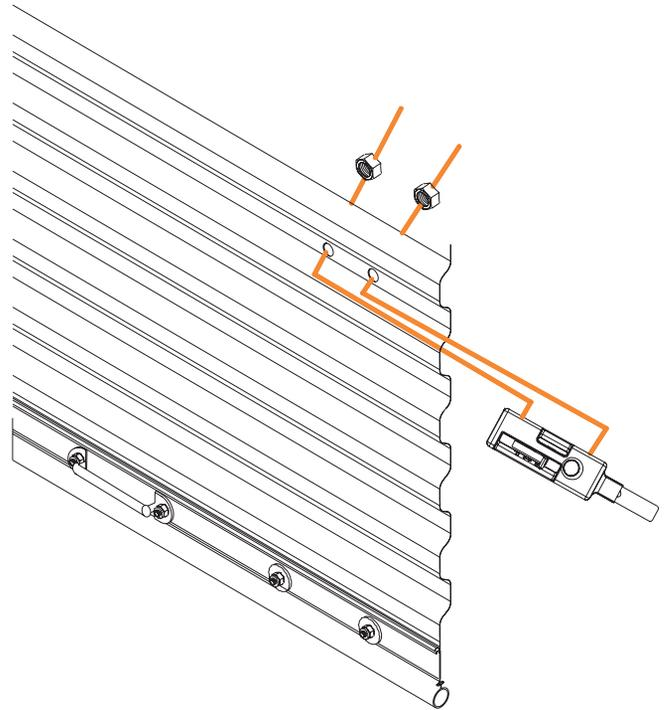
**E** Slide head stop from outside to inside of each mounting bracket.
