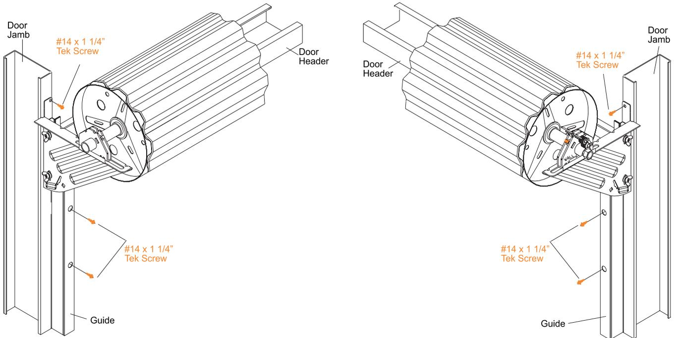
**B** The opening edge of guides should be inset a very small amount (about 1/8 inch) from the door jamb opening on each side to minimize the potential of hitting the guides when entering through the door opening. Both guides must be plumb and level with each other. *NOTE:* If jambs are installed correctly, the outside to outside measurement of guides should be approximately 1 inch wider than the curtain width.
