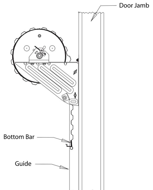
**D** Install the Slide Lock with hardware provided.
