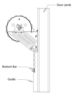
**D** Install the Slide Lock with hardware provided.
