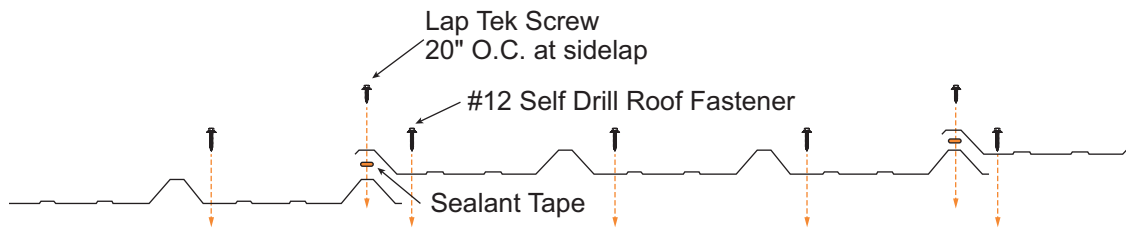
"R" and "PBR" Roof Panel Fastener Spacing, Intermediate Purlins, Girts, Eave Strut
