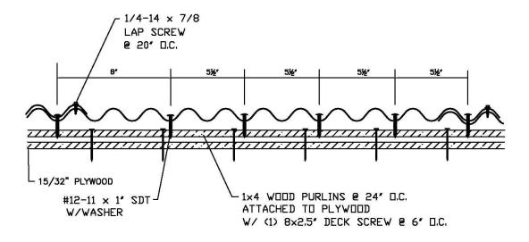
Figure 1. Fastener Pattern A and Fastener Pattern B
