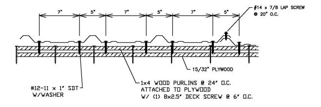
Figure 1. Fastener Pattern A and Fastener Pattern B
